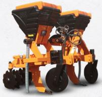
A versatile, multi-action implement for subsoiling, fertilizing, and cultivating sugarcane cultivation. It has discs for cutting straw, a subsoiling rod and an incorporating harrow. The implement also acts as a furrower/fertilizer, removing the harrow kit and screwing the handles on the rods that come with the equipment.
