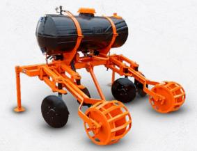
Implement used to cover the sugar cane stalks in the planting rows, with 2 rows working simultaneously. Defensive application in the furrow prior to covering. It has a set of concave discs with adjustable spacing and working angle. It also has compaction rollers for better contact between the soil and the stalks, avoiding air pockets and helping the efficient growth of the sugar cane.
