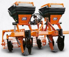
A versatile multi-action implement for subsoiling, fertilizing, and cultivating sugarcane cultivations. It has discs for cutting straw, a subsoiling rod, covering discs with working angle adjustment, and a crushing roller. The implement also acts as a furrower/fertilizer.
