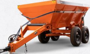
Equipment for distributing limestone and dry organic fertilizer, hydraulically driven, with belt system and centrifugal distribution. Easy coupling and tandem axle for stability on uneven ground.
