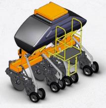
It carries out the fertilization of sugarcane stalks, mainly when harvested raw and mechanically. It has four applicator sets composed of one 26-inch straw cutting disc, two 18-inch mismatched flat discs with a deep fertilizer applicator, and two rubber wheels that close the straw cutting.
