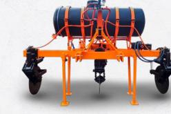
This equipment was developed to apply fertilizer in the rows of sugarcane ratoon, aimed at controlling pests. Ratoon cutting is mainly carried out in sugarcane fields, which have a high incidence of soil pests, and increases efficiency in managing them. Equipped with a 6x4 toolbar, the implement works with 3 rows simultaneously. It has discs for straw cutting and a device for injecting crop protection products beneath the soil.
